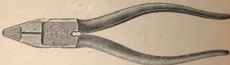
FIG. 244.—Combined side cutting pliers and wire connectors.
